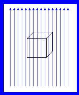
Key here is flux through the bottom (coming into box bottom = -ve [<0] flux outward from bottom)
