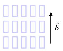
Dipoles of the molecules orient along an externally applied electric field. Change the field → change the birefringence → change the polarization of transmitted light → pass through polarization analyzer to change the intensity
