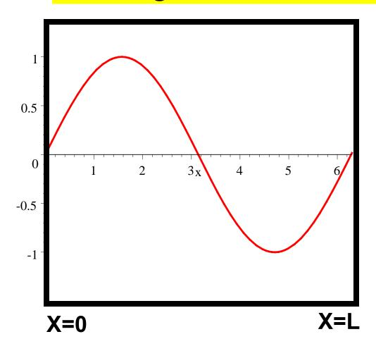
A sinusoidal E&B wave can exist in a metal box if the E field is ZERO on the boundary of the box. This requires the wave to be zero at x=0,L. This is possible if,
