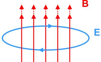
If there is a changing magnetic field, then there will be electric fields induced in closed paths. The electric fields direction will tend to reduce the changing B field.
