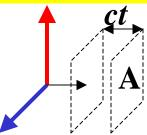
Suppose we have transverse E and B fields moving, at velocity c, to the right. If the energy density is 2 and the field is moving through are  $u = \varepsilon_0 E^2$  and the field is moving through area A at velocity c covers volume Act,
