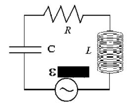
• As frequency is changed from resonance, either up or down,  $(X_L-X_C)$  no longer is zero and  $\mathbb{Z}$  must therefore increase.
