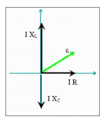
Since power peaks at the resonant frequency, try to get  $X_L$  and  $X_C$  to be equal. Power also depends inversely on R, so decrease R to increase Power.
