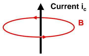
If there is a changing electric field through the loop, then there will be magnetic fields induced about a closed loop path.
