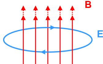
If there is a changing magnetic field, then there will be electric fields induced in closed paths. The electric fields direction will tend to reduce the changing B field.
