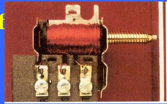
Magnet off → plunger held in place by spring Magnet on → plunger expelled → strikes bell
