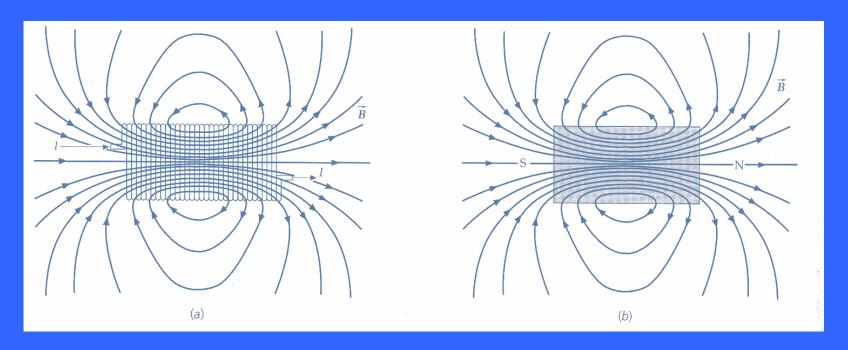
The big difference is that we can turn the solenoid on and off! It attracts/repels other permanent magnets; it attracts ferromagnets, etc.
