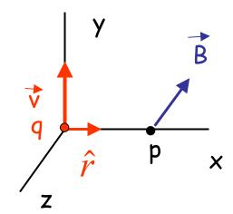
$$\vec{B} = \frac{\mu_0}{4\pi} \frac{q\vec{v} \times \hat{r}}{r^2} \qquad \qquad \mu_0 = 4\pi \times 10^{-7} \text{ T} \cdot \text{m/A}$$
