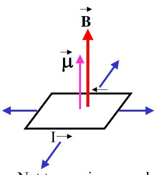
Net torque is **zero** when B is parallel to  $\mu$
