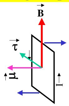
Net torque is **maximum** when B is perpendicular to  $\mu$
