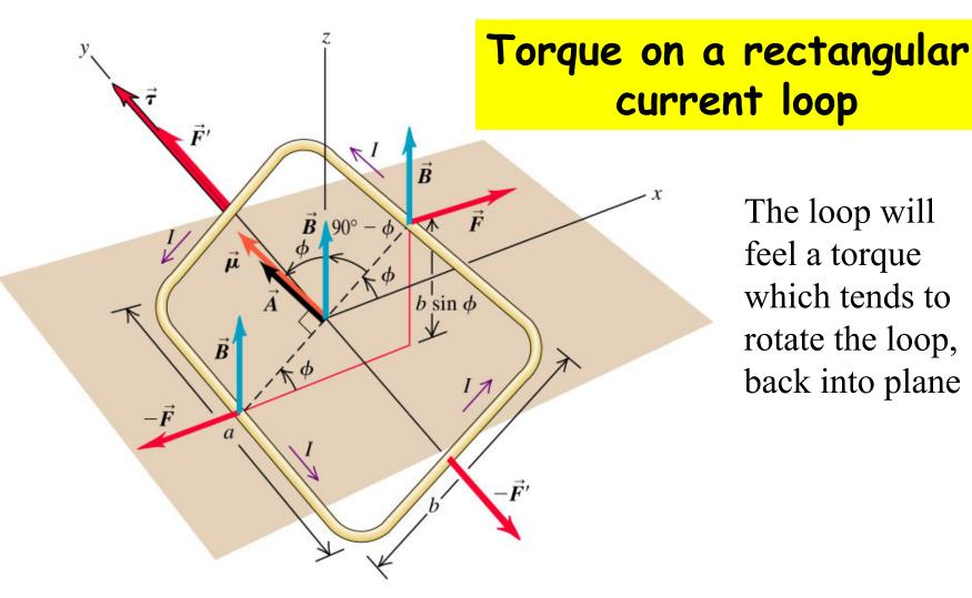
The loop will feel a torque which tends to rotate the loop, back into plane
