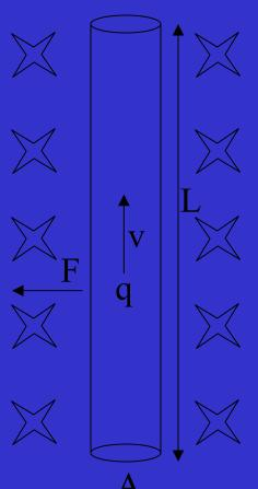
Suppose we have a straight wire with current where charges q are moving upwards and there is a B field pointing into this slide. There is a  $\vec{F} = q\vec{v} \times \vec{B}$  force tending to push the wire to the left.
