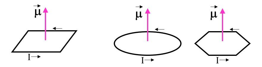
For any shape,  $\mu$  = current×area= I A and  $\vec{ au} = \vec{\mu} imes \vec{B}$
