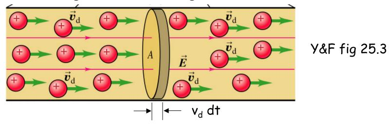
Current Density, J, is the current flow per unit area  $(amp/m^2)$
