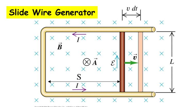
The area is LS(t) and dS/dt equals velocity of slider
