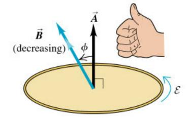
Positive flux  $(\Phi_B > 0)$ Flux becoming less positive  $(\frac{d\Phi_B}{dt} < 0)$ Induced emf is positive  $(\mathcal{E} > 0)$
