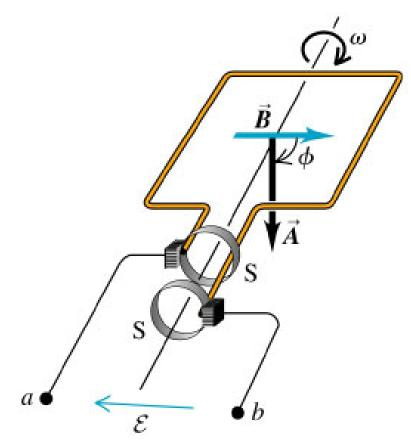
Wire loop area A rotates with respect to constant magnetic field.
