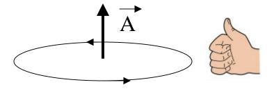
The choice of vector A direction defines the direction of EMF with a right hand rule. Your thumb in A direction and then your fingers point to positive EMF direction.
