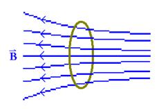
When the loop is stationary: the flux through the ring does not change!!!  $\Rightarrow d\Phi/dt = 0 \Rightarrow$  there is no emf induced and no current.
